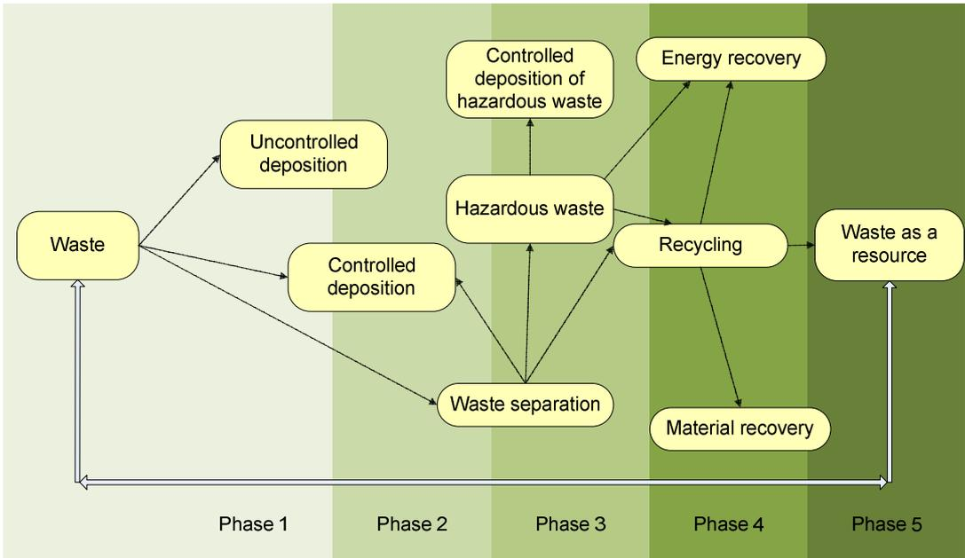
Fig. 5: Phases of waste management development (Source BMZ Resource waste, 2012)
