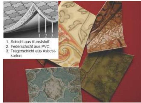
Figure 4: Asbestos cushion vinyl floor tiles/sheeting (Source ETI)
